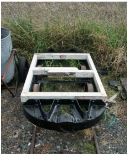
Chassis with newly fitted wood.
